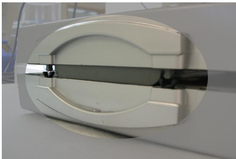
Figure 6: Place the top anode plate on top of the gel sandwich, making sure the locking mechanism is correctly positioned.
